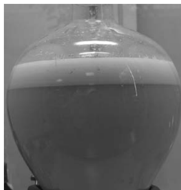
Fig. 2. Direct contact two phase emulsion after four days left in repose in a separation funnel.
